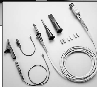
TDS 220 Digital Real-Time Oscilloscope (top); P5100 High-Voltage Probe (right).
